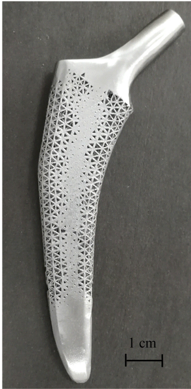
Fig. 12 Titanium-based alloy implant with optimized lattice architecture built via SLM
